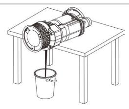
The oil volume for the models which are not included in the tables: about 80% of the total oil cylinder capacity (theoretically, the oil level should cover the mating ring).
