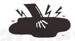
To prevent water from entering inside the cable, be sure to securely mold the cable connection portion.
