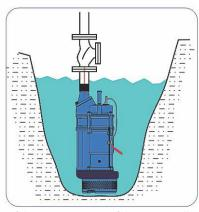
If the water capacity of the pit is small, in order to avoid frequent start-ups, a rubber ball check valve should be installed at the outlet junction. Also move the electrode up as far as possible.
