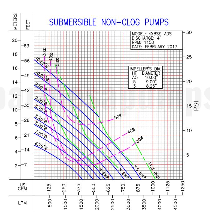
Testing is performed with water specific gravity of 1.0 @ 68 °F (20 °C); other fluids may vary performance.
